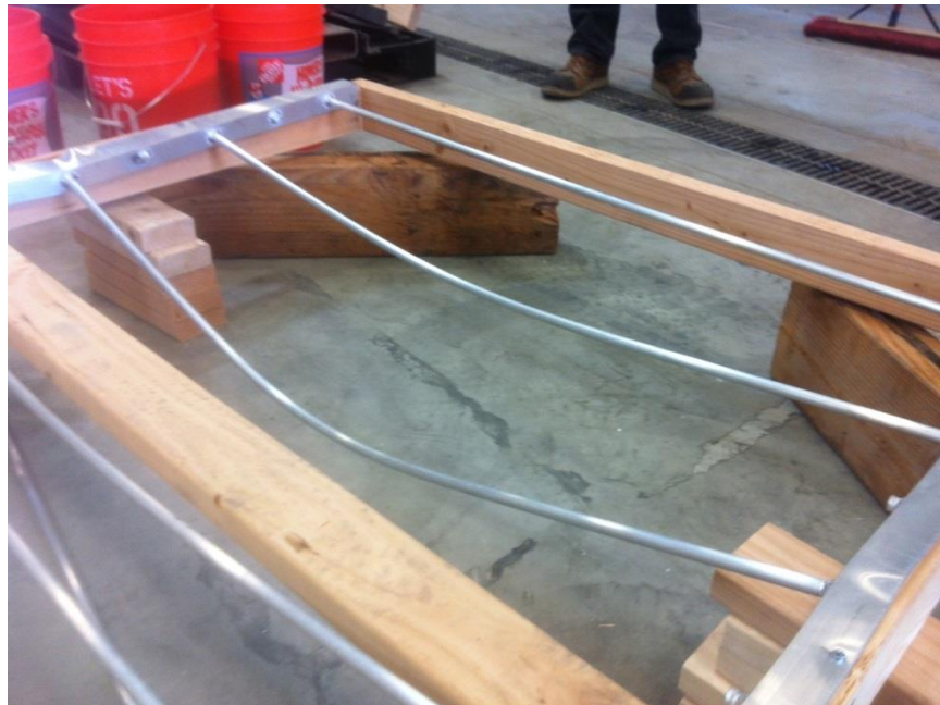
Photo No. 6 Test Specimen #3 after 200 lb. dynamic impact from 48"
