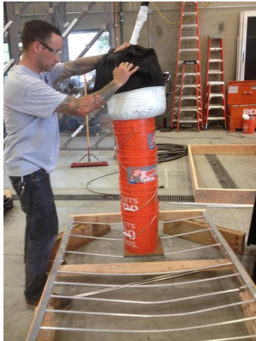
Photo No. 5 Test Specimen #3 during 200 lb. static test
