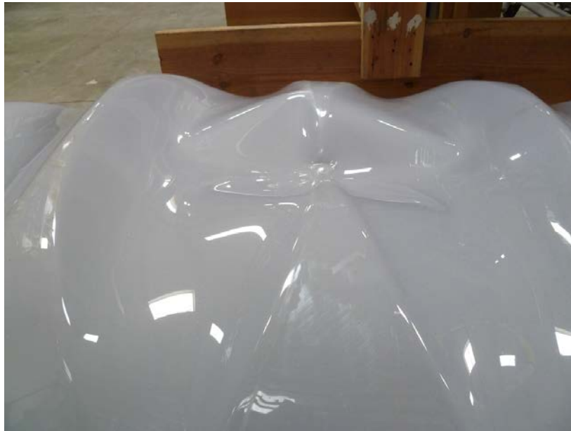
Photo No. 2 OSHA Safety Drop Test After Load Applied – Inversion of Dome Ridge
